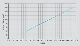
$\Delta T$  between reference ambient temperature and average water temperature = 10 K 103 W/m² (in accordance with EN14240)
