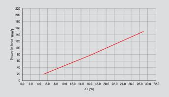
$\Delta T$  between mean water temperature and reference room temperature = 15 K **71 W/m²** (in accordance with EN14037)
