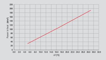
$\Delta T$  between mean water temperature and reference room temperature = 15K **96 W/m²** (in accordance with EN14037)
