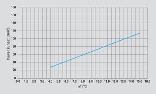
$\Delta T$  between reference ambient temperature and average water temperature = 10 K  $74~W/m^2$  (according to EN14240)
